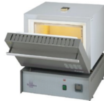
A common muffle furnace. Note the thick insulating layer on the inside to prevent overheating of the exterior
