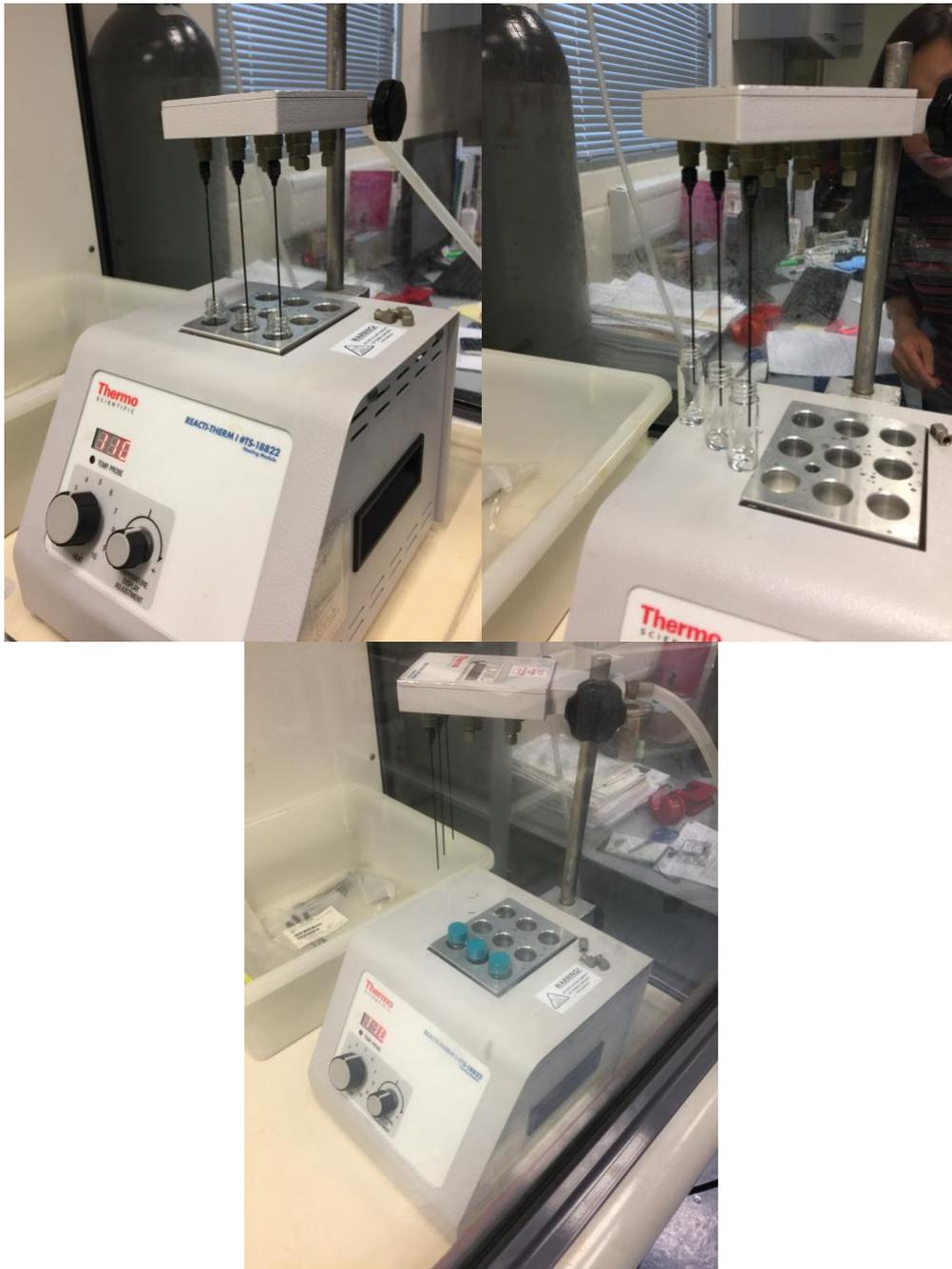
Figure 4 – Drying in and out of the block / heating in the block. Note, for all steps BUT the first dry down, the vials are dried at room temp (second picture, not in the heated block).
