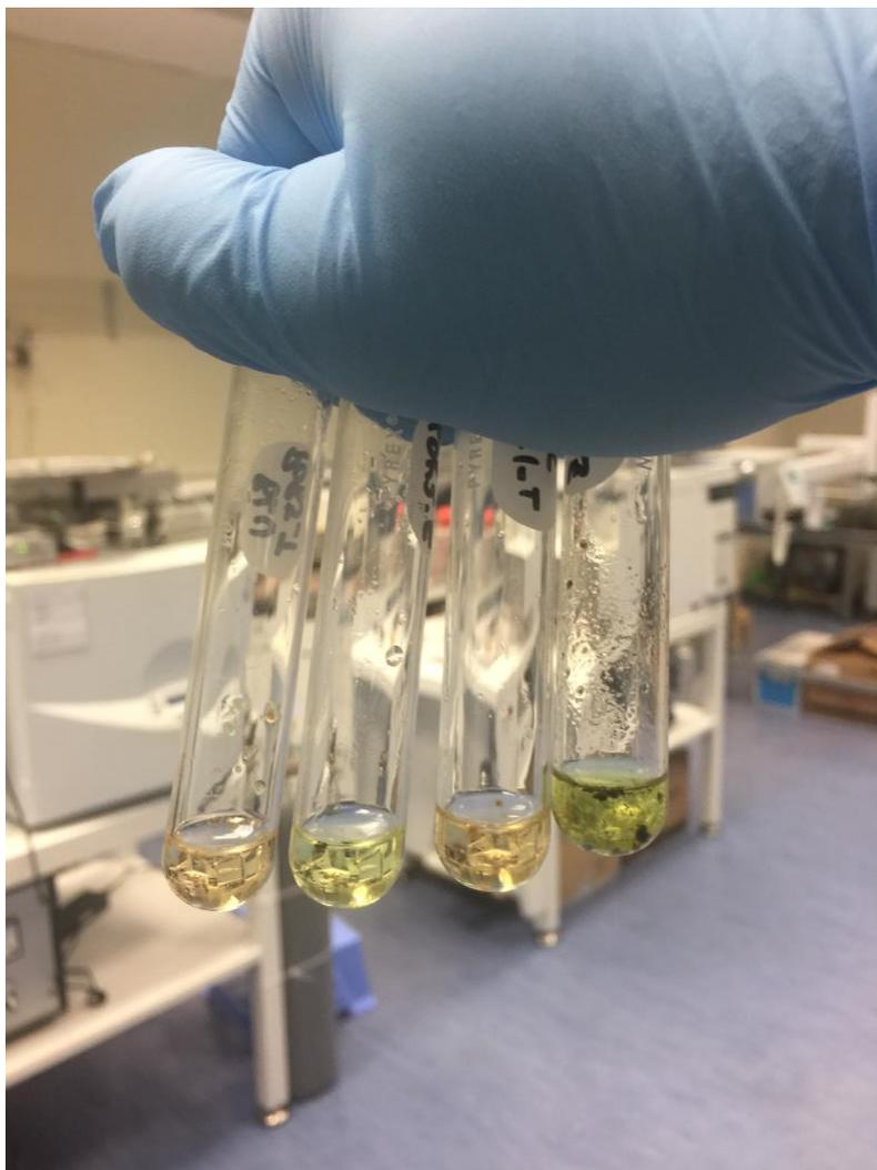
Figure 1 - Hydrolysate after 20 hours. Note, some samples may be clean (left two) or “dirty” (right two) – remnant material. These will need to be filtered and (likely) Dowex purified.
