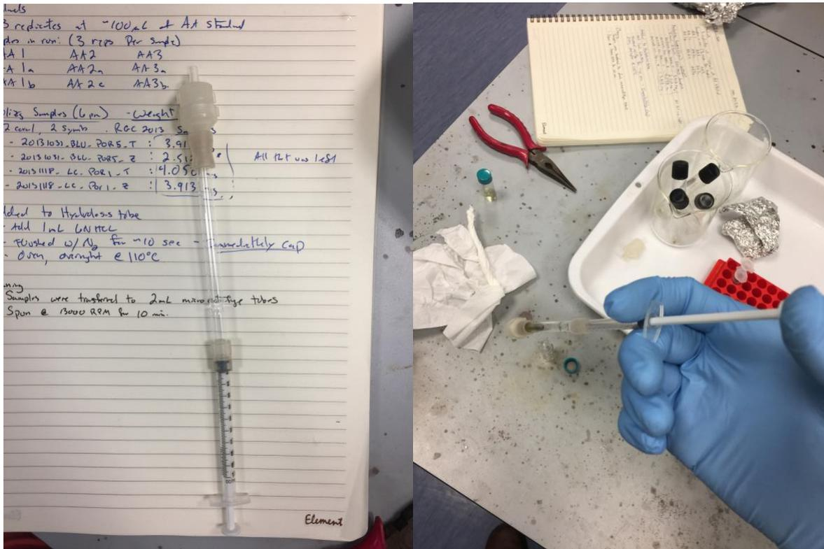
Figure 2 – Filter setup. After hydrolyzation, suck up sample with just broken glass pipette, then attach filter tip, then pass through filter into vial.
