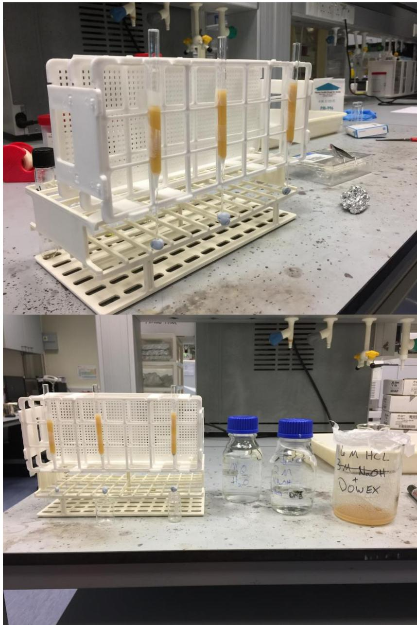
Figure 3 – Dowex ion-exchange column set up.
